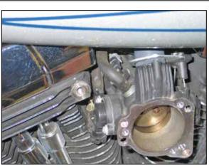
6. On Models equipped with the electrical pigtail, using the provided tie wrap, secure the wiring pig tail to the throttle body wiring harness.
