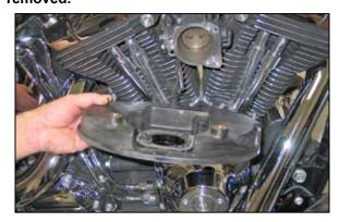
Remove the air filter base from the throttle body and unhook the wiring pig tail from the filter base.
